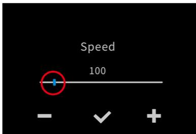
Click "+" or "-" or drag the slider to adjust the printing speed. Click "√" to confirm and back to the previous screen.
