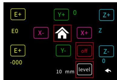
Moving-axes Screen: click the corresponding axis icon to move the axis, click the central house icon to home all the axes, and click "level" to start auto-leveling. Click off to unlock the motor.
